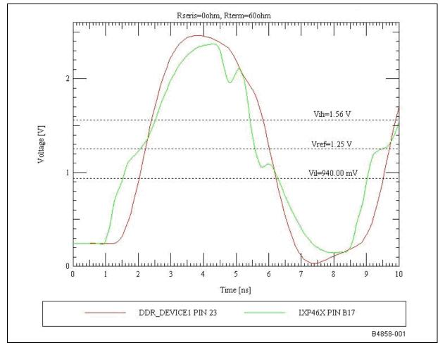
The simulation results in Figure 48 are for the RAS circuit, the voltage waveform meets the DDR device input voltage requirements.  $V_{il(max)}$  of  $V_{ref}$  – 0.310 or 940 mV and  $V_{ih(min)}$  of  $V_{ref}$  + 0.310 or 1.56 V are easily achieved at the receiver (DDR\_DEVICE1). The receiver waveform must also not exceed a maximum voltage of  $V_{in(max)}$  = 2.8 V or the minimum voltage of  $V_{in(min)}$  = -0.3 V.
